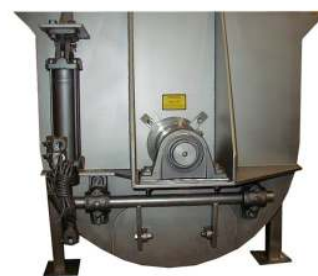
End Discharge Gate
