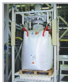
Automatic bag loop release.
