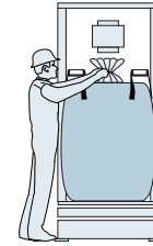
8. Bulk bag spout removed from filling nozzle and tied.
