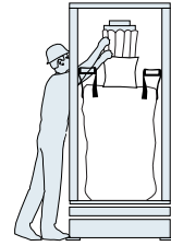
3. Liner or bag spout is attached to inflatable neck seal.
