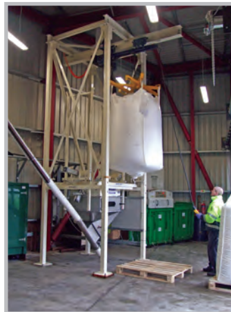
3. Traversing bag into position
