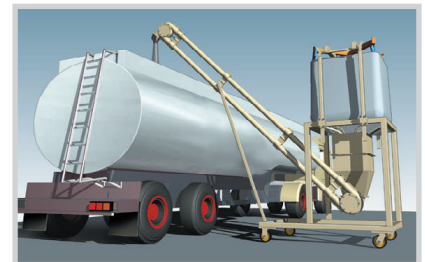
A bulk bag discharger & an AMC load a road tanker truck.
