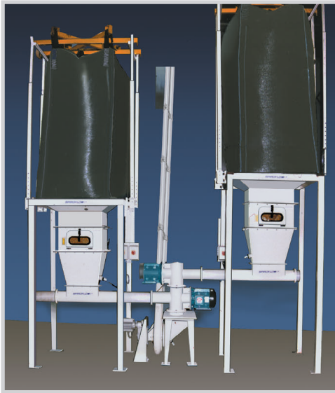
An AMC elevates material from a transition hopper fed by two bulk bag dischargers via spiral conveyors.
