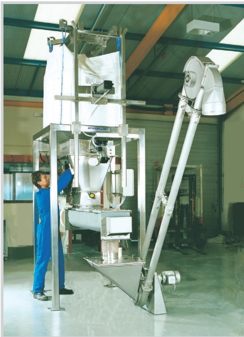
This AMC is designed for handling titanium dioxide. The aero mechanical conveyor is the only effective method of handling this type of product.
