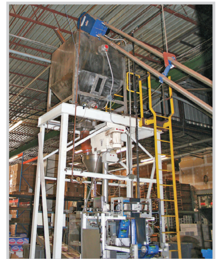
An AMC transfers flavored coffee powder from a blender up to a packing machine.
