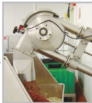
Interlocked inspection hatch in sprocket housing.
