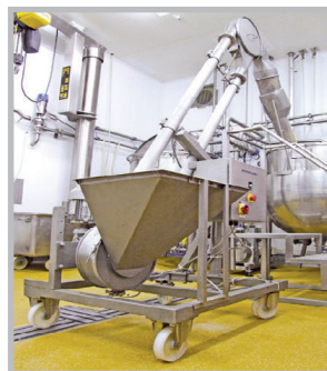
An AMC with a simple bag dump hopper for non-dusty materials.
