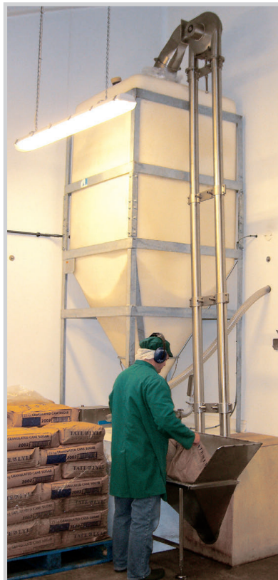
An around the corner Aero Mechanical Conveyor feeds chemicals to a mixing vessel.
