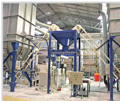
Two (2) AMCs deliver tin oxide from process to packaging.
