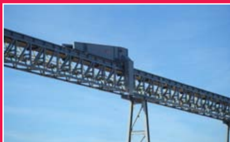
A traveling tripper with side discharge works well for filling large bulk storage areas.
