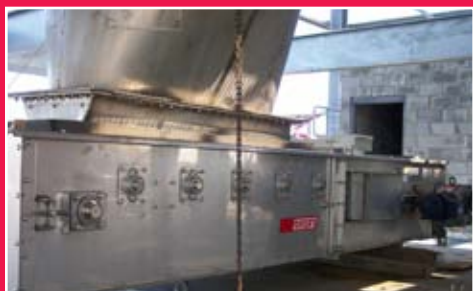
Stainless steel conveyor housing with stainless bearings and shafts are available for highly corrosive applications.
