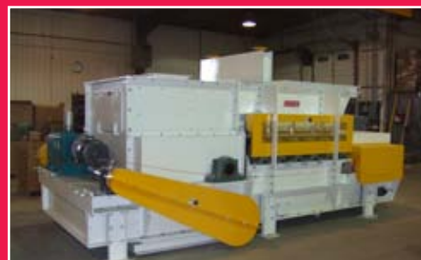
A large custom coal feeder is assembled, tested and readied for shipment.
