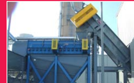
Steep incline, dual chain drag conveyors provide positive conveyance for bulky, difficult to handle products such as wood waste.
