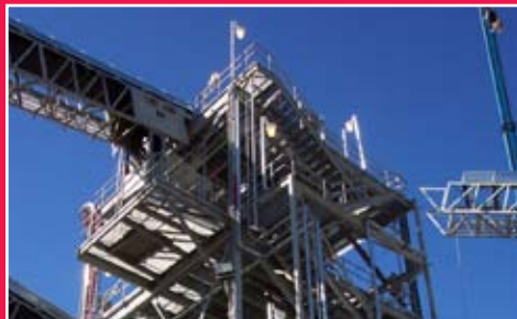
Our conveyor system accessories include structural transfer towers, transition chutes and trusses with catwalks and handrails.
