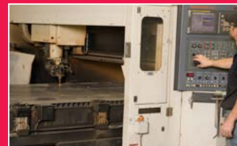
Our 4,000-watt laser has 3-D cutting capabilities and features an automatic feed table for around-the-clock production.
