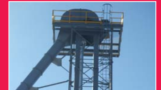
Bucket elevator shown with head service platform, handrail and custom discharge transition.
