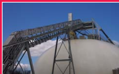
Our Series FLX conveyor uses a corrugated sidewall belt for conveying up steep inclines.
