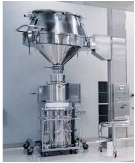
An inverted fluid-bed dryer bowl directly discharges into a Comil® U30 on a portable stand, feeding a stainless steel drum.
