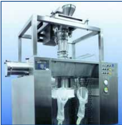
Quadro custom engineered this integrated milling solution incorporating the Comil ® with a Carlisle Extract crossflow system.
