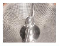
Keeps powder and fluid from entering the driven shaft.
