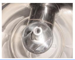
Specially designed grooves ensure no powder or cleaning solution enters any joints between metal parts.
