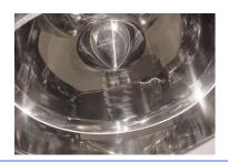
Cleaning fluids flow down the cone and drip from one point.
