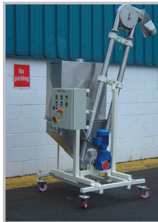
Mobile aero mechanical conveyors are used extensively both in and out of factory environments.
