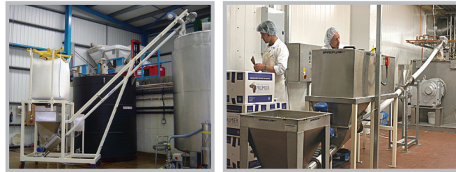
Mobile designs allow users to convey a variety of materials at multiple locations. Flexible screw conveyors can have multiple inlets and multiple outlets.
