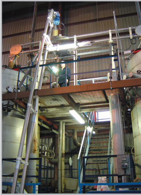
Aero mechanical conveyors are ideal for difficult products such as titanium dioxide and other products which have a tendency to smear and are cohesive.
