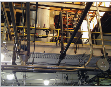
Multiple Cableflow conveyors move coffee beans from five silos to a high speed packaging machine at 10,000 lb/hr (4,500kg).
