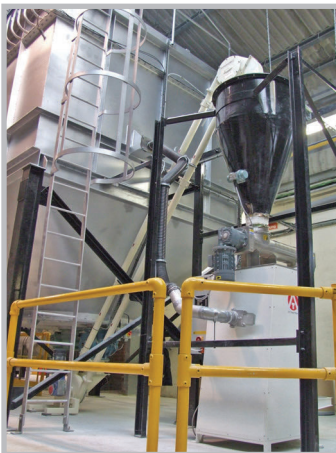
This aero mechanical conveyor is elevating chemicals to a hopper. Discharge heights can be specified for individual requirements.
