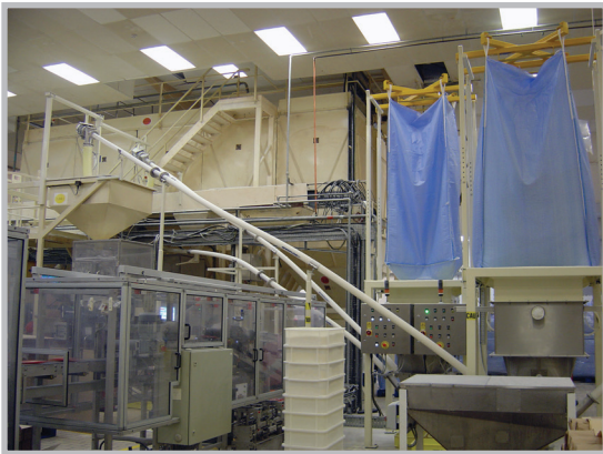
Mobile designs allow users to convey a variety of materials at multiple locations. Flexible screw conveyors can have multiple inlets and multiple outlets.
